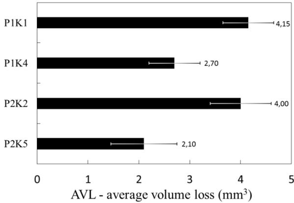
Figure 7: Volume weight loss – ASTM G65 (to be updated)
