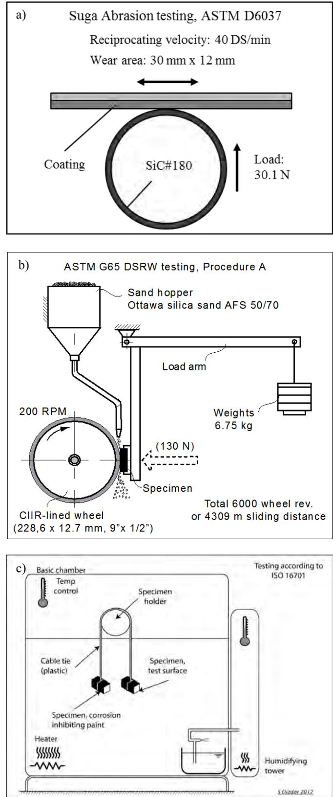
Figure 1: Wear resistance tests: a) ASTM D6037, b) ASTM G65 and c) cyclic corrosion test according to ISO 16701.
