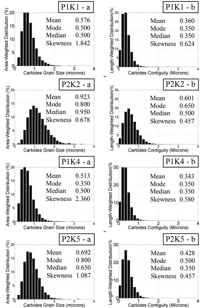
Figure 4: Respective weighted distributions of a) Carbides Grain Size (CGS) and b) Carbides Contiguity (CC)
