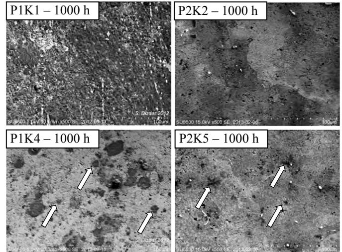
Figure 9: SEM micrographs (x500) of HVOF and HVAF coatings exposed to cyclic corrosion test after 1000 hours
