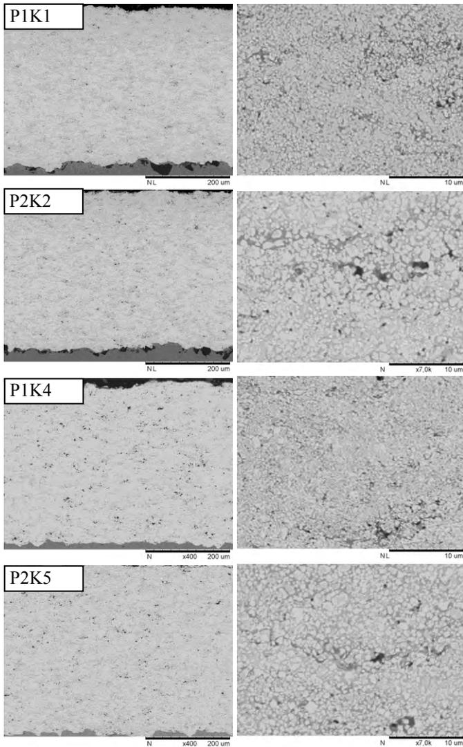
Figure 2: SEM micrographs of respective coating cross sections (X400- left; X7000-right)
