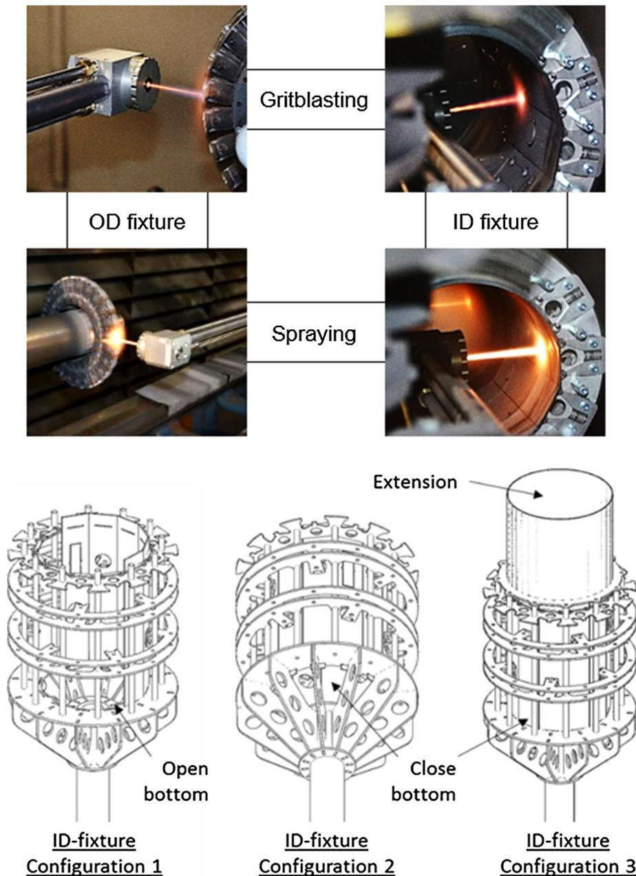
**Fig. 1** Specially designed outer diameter (OD) and inner diameter (ID) sample holder for ID-HVAF system
