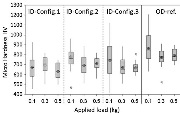
**Fig. 6** Boxplot representations of ASTM E384-10 microhardness values of  $\text{Cr}_3\text{C}_2\text{-NiCr}$  ID-HVAF coatings
