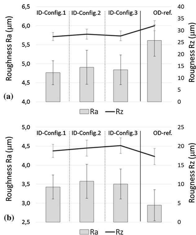
Fig. 9 2D Roughness measurements for (a)  $\text{Cr}_3\text{C}_2\text{-NiCr}$  and (b) WC-CoCr ID-HVAF-sprayed coatings
