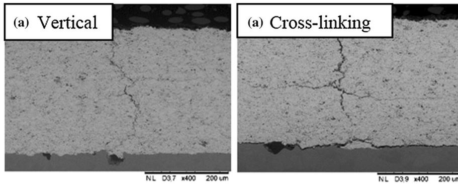
**Fig. 5** Crack patterns encountered for WC-CoCr coatings
