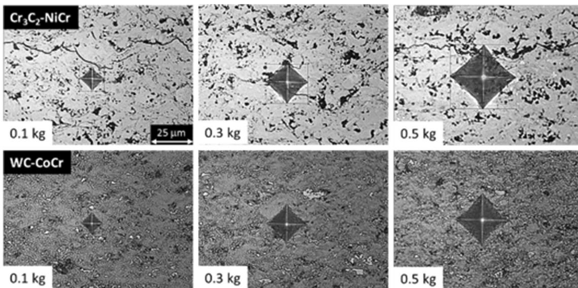
Fig. 7 Optical micrographs of Vickers indentations
