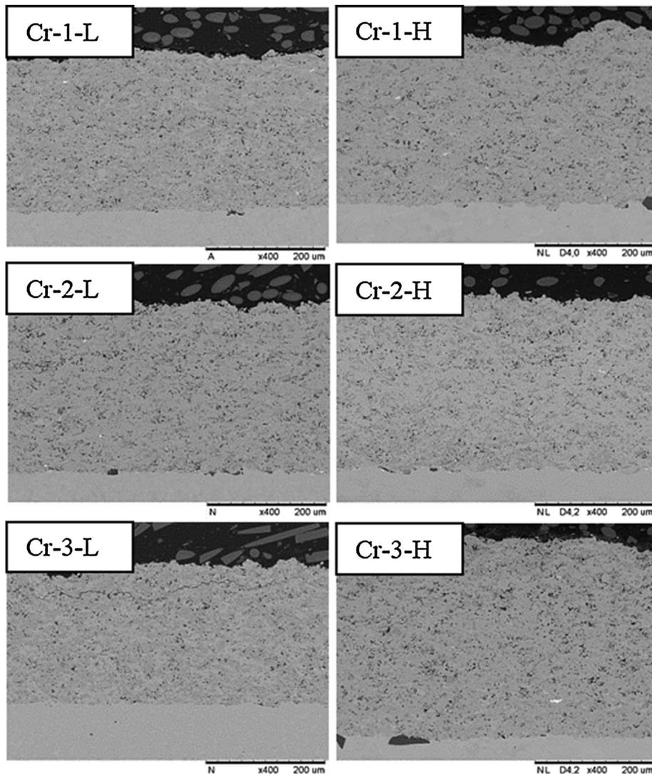
**Fig. 3** Cr<sub>3</sub>C<sub>2</sub>-NiCr coatings sprayed on ID sample holder
