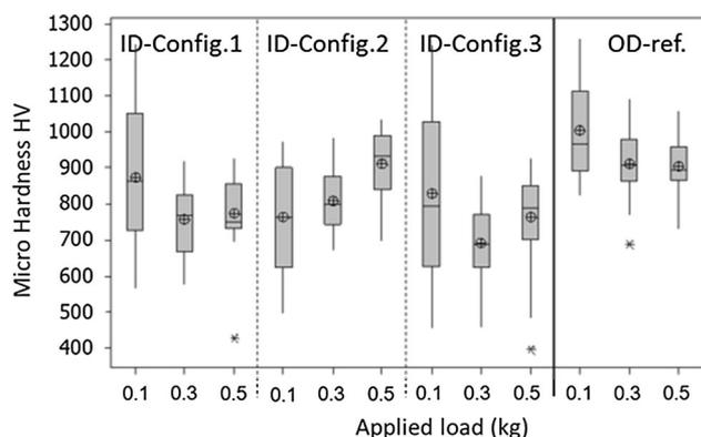
Fig. 8 Boxplot representations of ASTM E384-10 microhardness values of WC-CoCr ID-HVAF coatings
