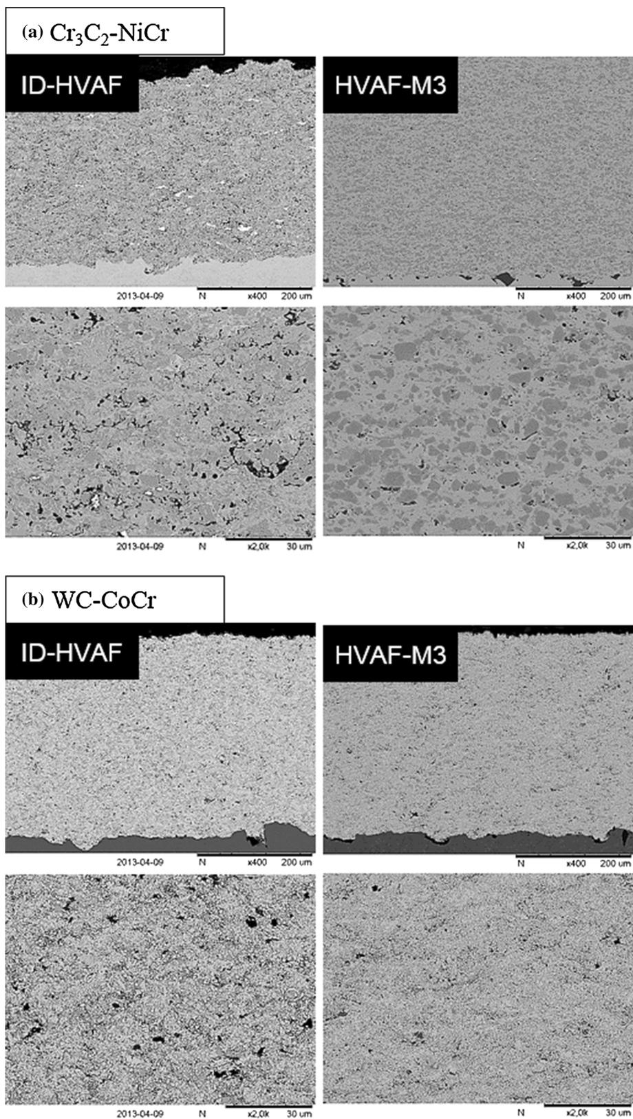
**Fig. 2** Comparison of coatings sprayed by ID-HVAF gun and HVAF-M3 system on OD sample holder for (a)  $\text{Cr}_3\text{C}_2\text{-NiCr}$  and (b)  $\text{WC-CoCr}$  feedstock materials
