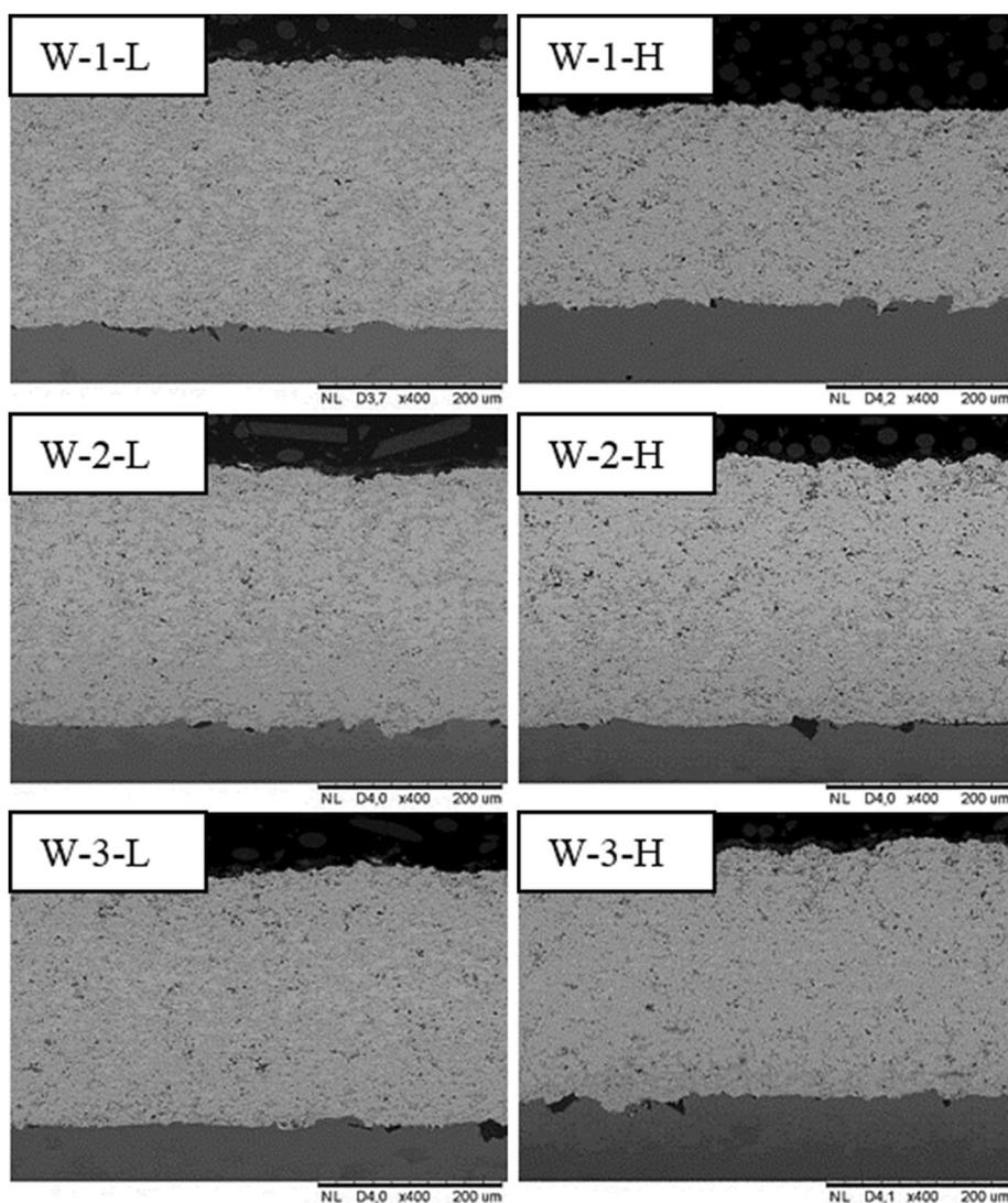
**Fig. 4** WC-CoCr coatings sprayed on ID sample holder
